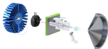
Figure 2 - Schematic of the Luxon ionization source
