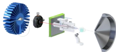
Figure 2 - Schematic of the Luxon ionization source
