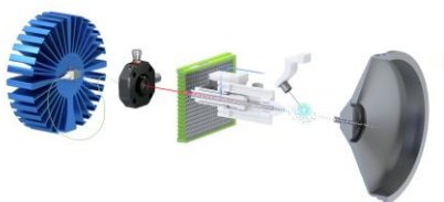
Figure 2 - Schematic of the Luxon ionization source
