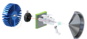
Figure 2 - Schematic of the Luxon Ionization Source
