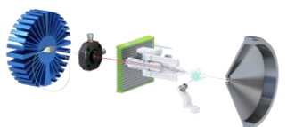
Figure 2 - Schematic of the Luxon ionization source
