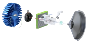
Figure 2 - Schematic of the Luxon Ionization Source
