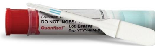
Figure 3 - Quantisal device for oral fluid sample collection
