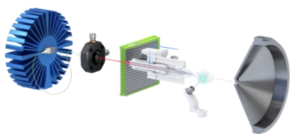
Figure 2 - Schematic of the Luxon Ionization Source
