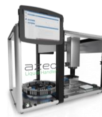
Figure 3 - Automated extraction system
