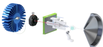
Figure 2 - Schematic of the Luxon Ionization Source
