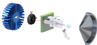
Figure 2 - Schematic of the Luxon Ionization Source
