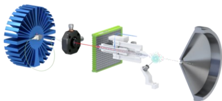
Figure 2 - Schematic of the Luxon Ionization Source
