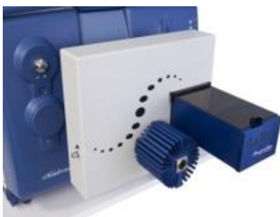
Figure 2 LDTD system on SCIEX 5500 Qtrap™ Mass Spectrometer
